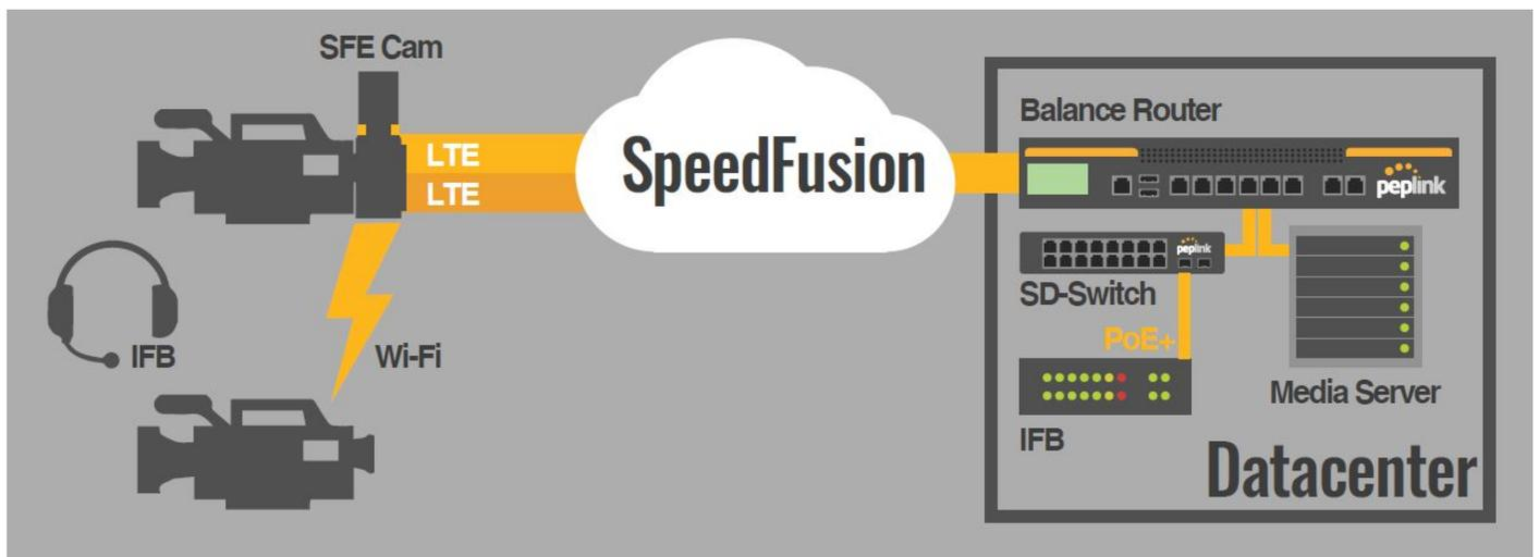
The following example shows how to set up a speedfusion connection between a SFE Cam and a Fusionhub. This process is the same for any Peplink router. SpeedFusion profiles can be configured using [InControl](#) or the local web admin interface.
