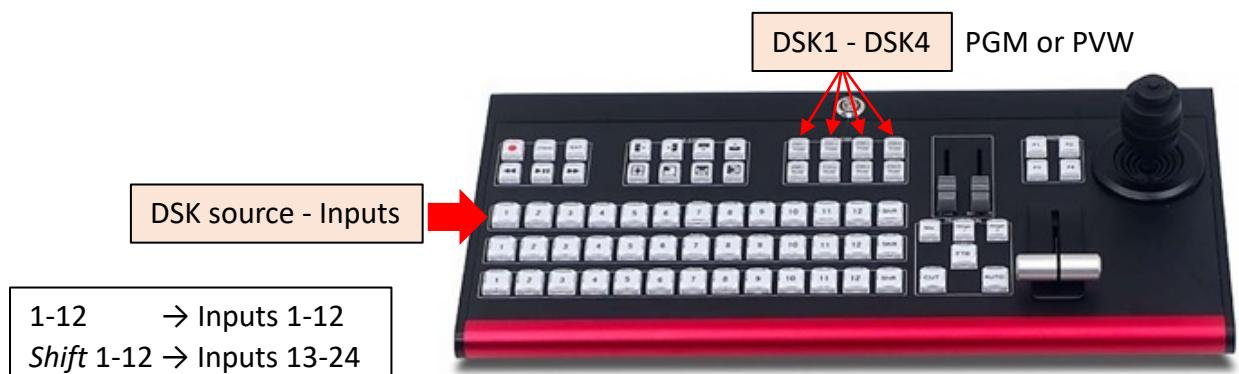
Press DSK1-DSK4 (PGM or PVW) to activate one of the downstream keys
