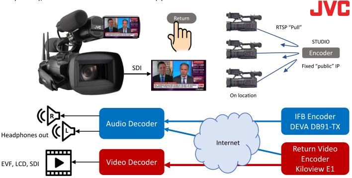
Return Video is displayed in the EVF/LCD and output via SDI when the pre-assigned button "Return Video" is pressed once. The second press would return the LCD/EVF/SDI to the live video output. The HDMI output does not switch to Return Video and outputs live video all the time. This allows using two monitors for simultaneous live and return video display.
