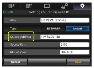
The Source Address is the "public" IP address of the encoder. The encoder installed at the studio must have fixed IP for cameras to "pull" the stream from. (Ports forwarding may be needed as well)
