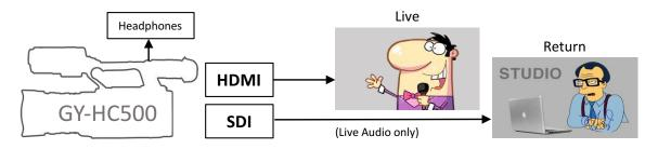
For Return Video we recommend the **Kiloview E1 H.264 encoder** and for the IFB - **DEVA DB91-TX** IP audio encoder. The camera can memorize up to 4 Return/IFB servers to allow quick switching between sources in the field via the camera menu.
