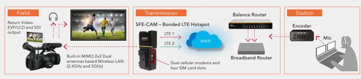
SFE-CAM is a bonded cellular hotspot that connects interactively to multiple GY-HC550/HC500 camcorders and features Peplink's patented SpeedFusion™ technology. SFE-CAM bonds multiple cellular and wireless LAN connections enabling the user to send digital video at greater speeds than you could with a single modem. Provided with dual cellular modems with redundant SIM slots and dual band Wireless LAN, you can use up to four different providers for bandwidth bonding.
