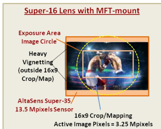
The illustration immediately to the left presents the exposure area (image circle) produced by attaching a Super-16 lens to the GY-LS300, using MFT adapter. Again, our interest is in a 16x9 framing and to eliminate any vignetting inside the 16x9 framing.
