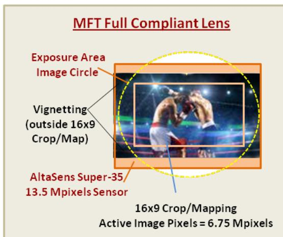
The illustration immediately to the left presents the exposure area (image circle) produced by attaching a fully compliant MFT lens to the GY-LS300. Again, our interest is in a 16x9 framing and to eliminate any vignetting inside the 16x9 framing.
