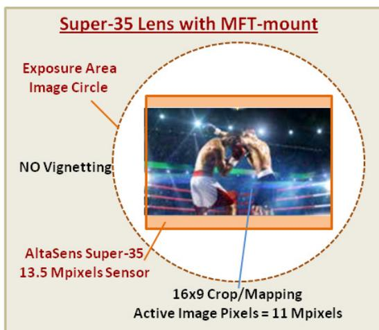
The GY-LS300 is designed to be a Super-35 format camera, with a native single Super-35 CMOS sensor with a total of 13.5 Mpixels (4512 x 3008) and an aspect ratio of 1.5. Any Super-35 lens with integrated MFT mount will expose the entire sensor, avoiding vignetting.
