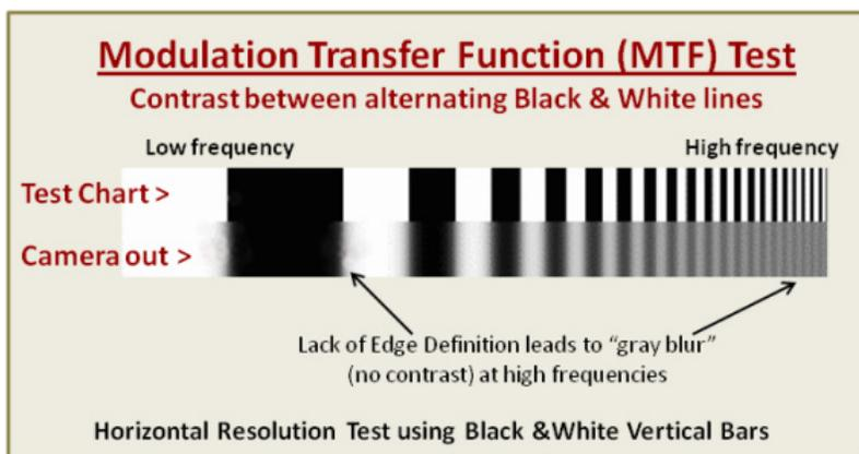
Such MTF performance is generally presented as a graph showing how the percentage of MTF declines as the frequency of alternating black and white lines increase. Let’s first look at a horizontal resolution test using black and white alternating vertical bars.
