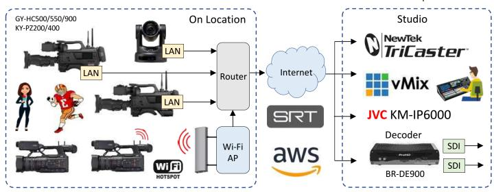
SRT protocol employs ARQ and FEC error correction and ABR (adaptive bitrate) to compensate for occasional data loss, latency, and jitter when sending video over unpredictable networks.
