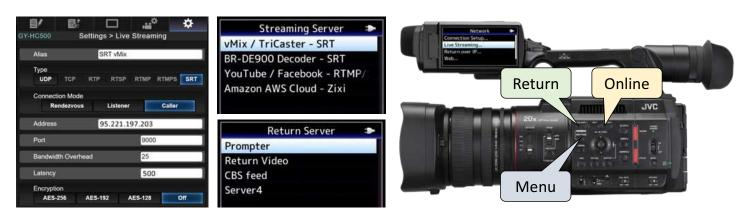
SRT protocol features real-time stream quality confirmation with the status displayed in the camera's LCD/EVF. When the receiver (decoder) detects the excessive data loss which cannot be corrected with the built-in error correction, the "LIVE" indicator will change color to notify the cameraman / talent that transmission quality may be compromised. Detailed stream quality data is available when pressing the "Status" button on the camera.
