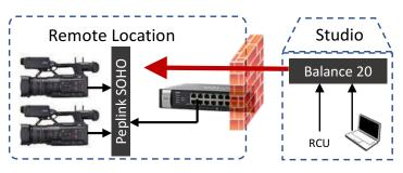
Placing the <u>Peplink Surf SOHO</u> **VPN Router** between cameras and the local router creates the "outgoing VPN" and allows to access cameras and other devices behind the firewall directly from the studio equipped with <u>Peplink Balance 20</u> (or other) VPN Host.
