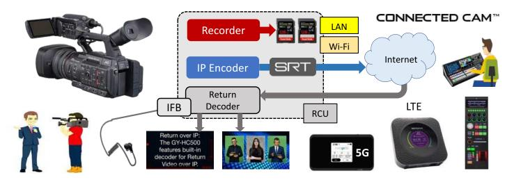
Setup on location is quick and simple: the camera can store 4 streaming destinations and return video (IFB) sources. With all settings pre-programmed, connecting to the Internet and pressing the "Online" button is all that is needed to start a contribution-quality video feed to the remote studio.
