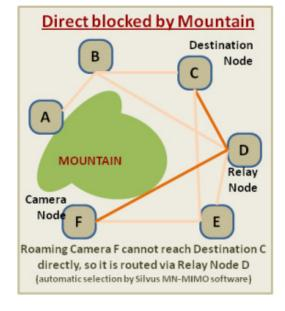
Every MESH Node is a radio transceiver, capable of transmitting, receiving, buffering, and forwarding data in UDP/TCP protocols over the IP-based private radio communications channel. The quantity of Nodes required to cover an event is of course subject to the size of the area, the local topography (is the area mountainous, hilly or relatively flat, or urban) and the extent of desired coverage. Buildings may impede connectivity, but also provide benefits in the form of RF reflections.
